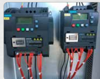
Head Feed and Spindle Variable speed controlled by two inverter Siemens SINAMICS V20
