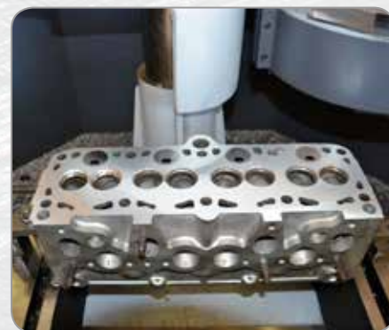
ALUMINIUM + STEEL PRE-CHAMBERS HEAD RESURFACING
