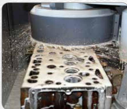
WET SURFACE GRINDING WITH COOLANT FLUID
