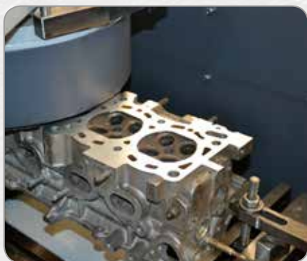
ALUMINIUM HEAD RESURFACING WITH TOOL
