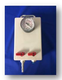
The FONDERA Model F2578 (photos to the left and right refer) has an additional feature in that it can do a leakdown test.
