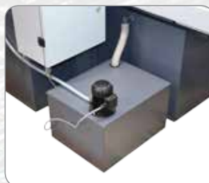
Cooling system complete of pump and tank
